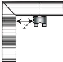
Use the hole on the top of the bracket to secure it using the provided screws (#2 Robertson).
